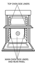
The surfaces of the oven liners are treated with a special vitreous enamel which absorbs cooking soils. At temperatures of 220°C (425°F) or above, the special surface enables these soils to be slowly destroyed. The higher the temperature the more effective it is.
